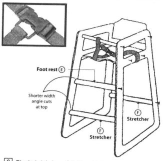
6 Check chair balance & tighten all bolts to complete assembly. Bolts can come loose over time. Bolts should be checked for tightness and retightened periodically.
