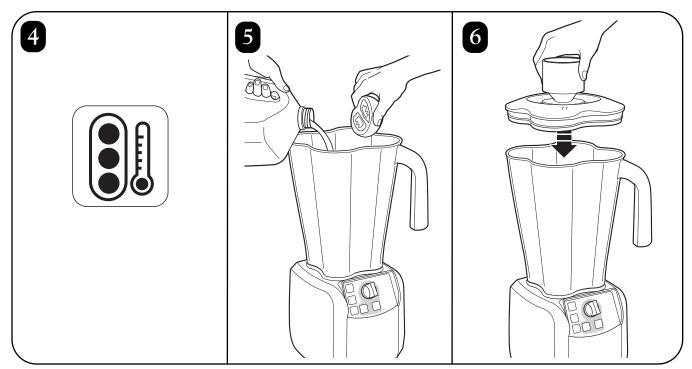
Temperature gauge alerts operator if motor overheats while blending back-to-back batches.
