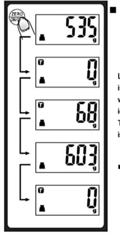
Condition 1: "ZERO" function When total sum of all loads on scale≤4% of scale's max.weight capacity. (4%=80g when capacity is 2000g; 200g when capacity is 5000g)
