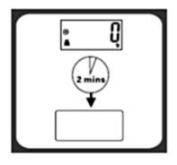
Auto shut-off occurs if display shows '0' or shows the same weight reading for 2 minutes.
