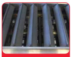
Step 13 - replace the pyramid radiants in reverse order (right to left), ensuring they are securely located on front and rear mounting tabs
