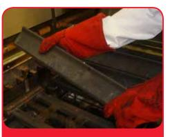
Step 8 - remove the radiants (left to right) and clean with a scourer and hot soapy water
