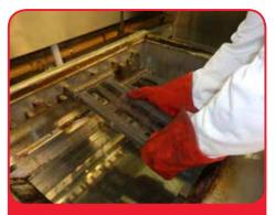
Step 9 - starting from left hand side remove burners (lift back of burner out first) and clean with dry scourer (do not immerse burners in water)
