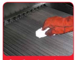
Step 3 - using a damp cloth, wipe any remaining debris from the bars
