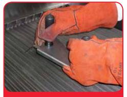
Step 2 - remove any food debris from the brander bars using the scraper.
