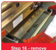
Step 16 - remove lower drip tray, clean in hot soapy water then replace. Remember to refill with water
