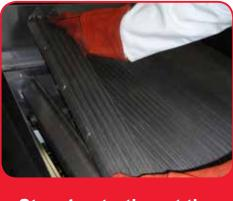
Step 4 - starting at the left hand side, use both hands to lift off the grill plates and remove from the unit
