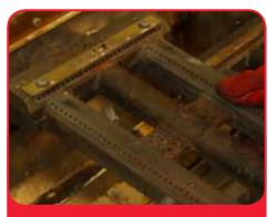
Step 10 - check jet holes and unblock as required (a paper clip is suitable but must be disposed of immediately after use)
