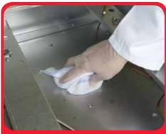
Step 7- Using a damp cloth wipe any spillages in chamber. Dry thoroughly.
