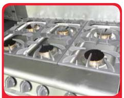
Step 8 - Replace hob panel, burner bases, burner heads and pan supports.
