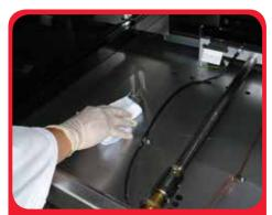
Step 5 - Clean oven base, sides and top with damp cloth. Dry thoroughly.
