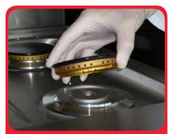
Step 3 - Remove burner heads. Clean with hot soapy water. Dry thoroughly.
