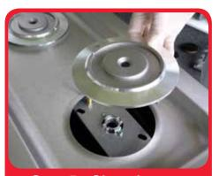
Step 5 - Clean burner bases in hot soapy water. Dry thoroughly.
